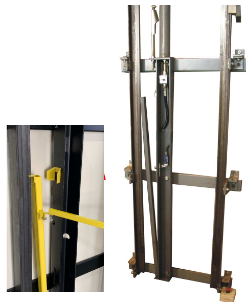
Image 5. Guides, pedestal and open prop unit.
