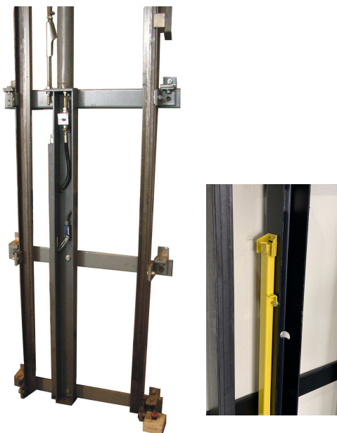
Image 4. Guides, pedestal and closed prop unit.
